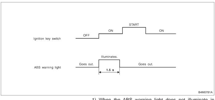
1) When the ABS warning light does not illuminate in accordance with this illumination pattern, there must be an electrical malfunction.
